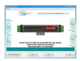
It is possible to use the program without connecting to the module, in this mode you can SAVE the configuration on your PC, which can then be sent to the QA-POWER-M at a later time.
