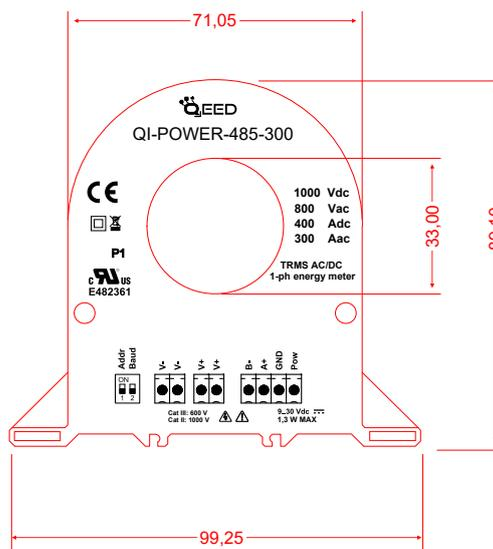
ANALIZZATORE DI RETE MONOFASE AC/DC - RS485 MODBUS QI-POWER-485-300
