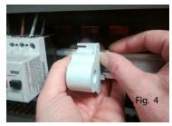
For mounting on DIN rail horizontally, once hooked on the bottom, push with both hands as shown in fig.3.
