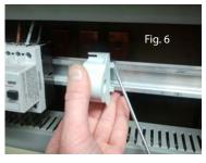
To release from DIN rail, use a screwdriver and lever up to release the fins (Figure 5 or Figure 6)
