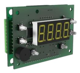
Universal module for controlling temperature, cooking times, cycles and processes.
