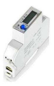
The QC-PM485 module is a single-phase power meter with direct insertion up to 100A, it is equipped with a backlit display and an RS485 serial port that communicates in Modbus RTU.
