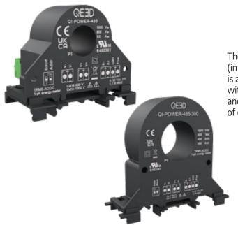
The QI-POWER-485 (in its 3 current sizes 50, 100 and 300A) is a single-phase network analyzer with direct measurement of both AC (TRMS) and DC current and energy without the need of external CTs.
